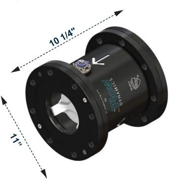
For best results install the Smart Valve downstream of water meter and backflow preventer (if present), but before any other equipment such as a pressure reducer or booster pump. Where possible it is recommended (but not critical) to have 10 diameters of pipe between the water meter and the valve. All flanged installations to use gaskets at each flange.
